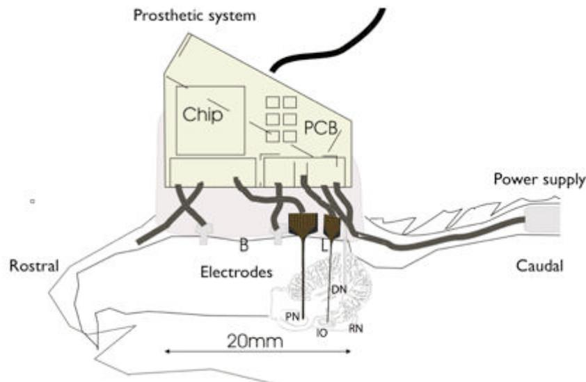
Figure 8. Design for a cerebellar neuroprosthetic prototype. An integrated computational system emulates the circuit properties of the cerebellum based on a theoretical model. This emulated cerebellar micro-circuit is interfaced to the input and output structures, the Pons (PN) and Inferior Olive (IO) and Deep Nucleus (DN) respectively. This paradigm has been successfully applied in in vivo replacement experiments [47]. Adapted from [45].
